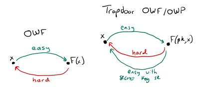
Figure 1: A one-way function (at left) is hard to invert on random inputs. A trapdoor oneway function/permutation (at right) is a function keyed by a public key. The function is easy to invert given the secret key and is hard to invert otherwise.
